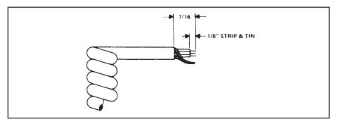
Fig. 2. Microphone Cable Preparation
