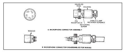
Fig. 3. Microphone plug wiring.
